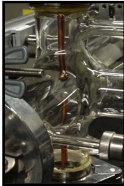
Figure 5.11: Photograph of sphere-to-sphere, copper electrode setup (electrode diameter = 7.5 mm, discharge gap = 1 cm)
