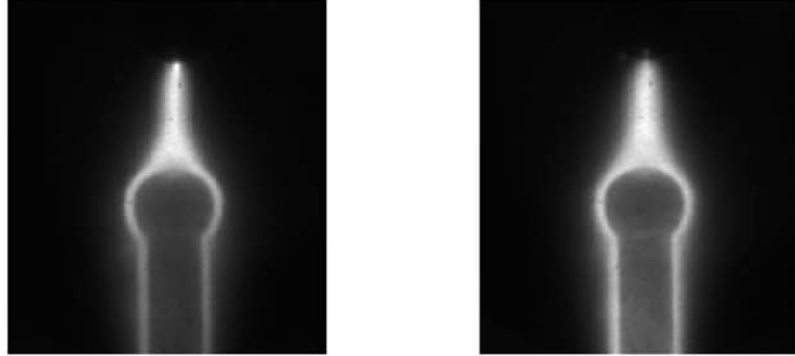
Figure 5.17: Broadband plasma emission ICCD images in helium ( P=100 torr, 100-pulse average, 200 ns ICCD camera gate). Left: Primary pulse, Right: Secondary pulse. From reference [53].
